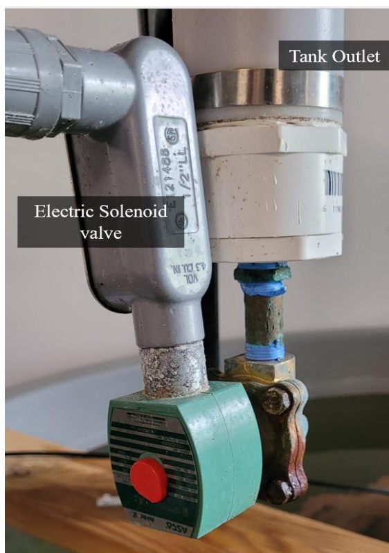
Figure 4. Electric solenoid valve to regulate release of artemia into larval fish tanks
