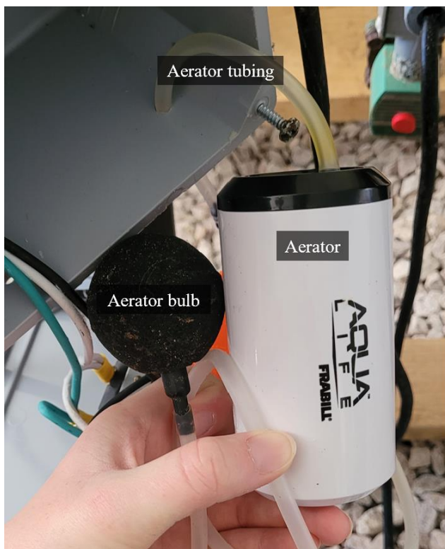
Figure 3. 110-volt aerator used to keep artemia alive throughout the day in the roto-mold holding tank prior to release into a larval fish tank
